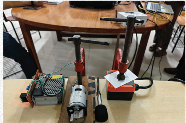
Fig. 2 Initial developed system for ground vibration data and Calibration Device (Known Frequency)
